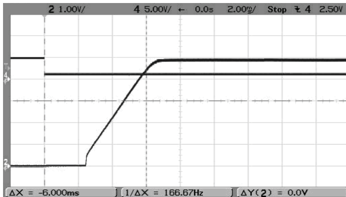
On/Off Enable Startup Delay (VIN=12V, Vout=5.0V, Iout=3A, Load=0) Trace 4=Enable In, Trace2=Vout
