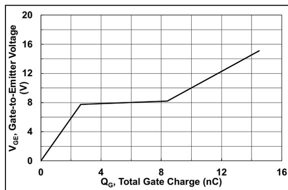
**FIGURE 5-4:** Typical Gate Charge vs.  $V_{GE}$ .
