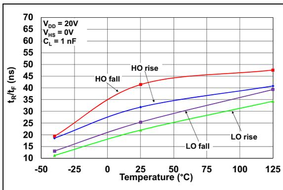
**FIGURE 2-27:** Rise/Fall Time vs. Temperature ( $V_{DD} = 20\text{V}$ ).
