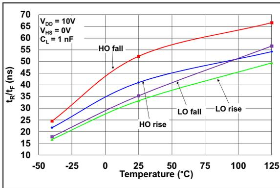
**FIGURE 2-26:** Rise/Fall Time vs. Temperature ( $V_{DD} = 10\text{V}$ ).
