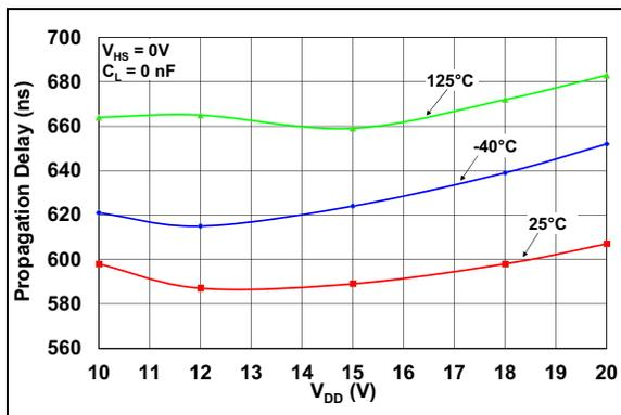
**FIGURE 2-33:** Overcurrent Propagation Delay vs.  $V_{DD}$  Voltage.
