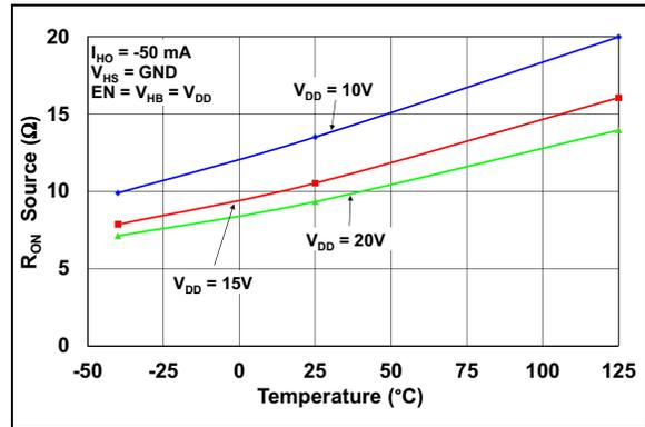
**FIGURE 2-16:** HO Output Source ON-Resistance vs. Temperature.
