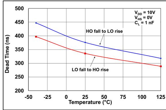
**FIGURE 2-29:** Dead Time vs. Temperature ( $V_{DD} = 10\text{V}$ ).
