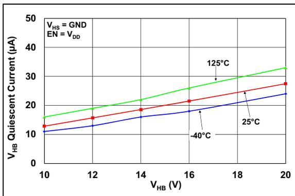
**FIGURE 2-3:**  $V_{HB}$  Quiescent Current vs.  $V_{HB}$  Voltage.
