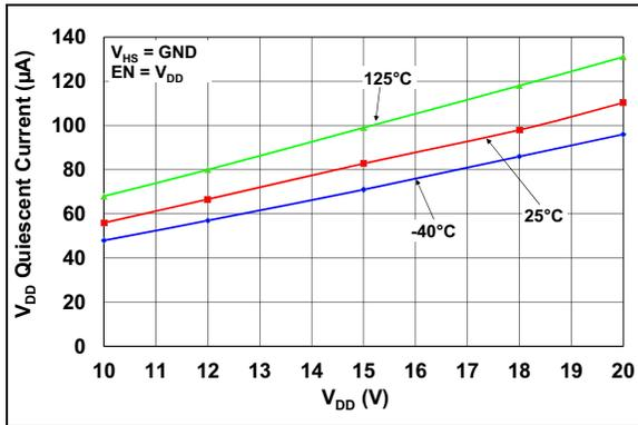
**FIGURE 2-1:**  $V_{DD}$  Quiescent Current vs.  $V_{DD}$  Voltage.
