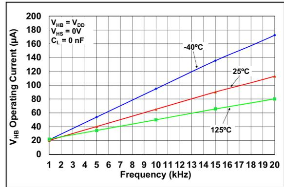
**FIGURE 2-10:**  $V_{HB}$  Operating Current vs. Frequency – One Phase.
