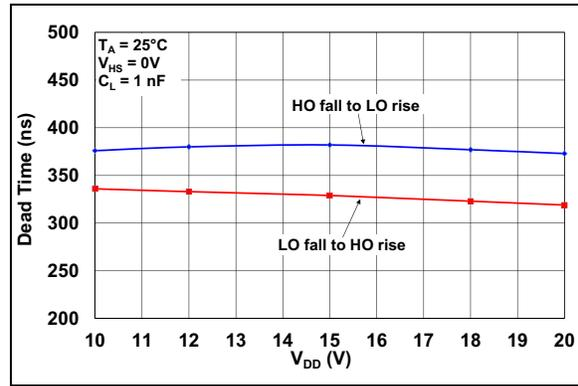
**FIGURE 2-28:** Dead Time vs.  $V_{DD}$  Voltage.
