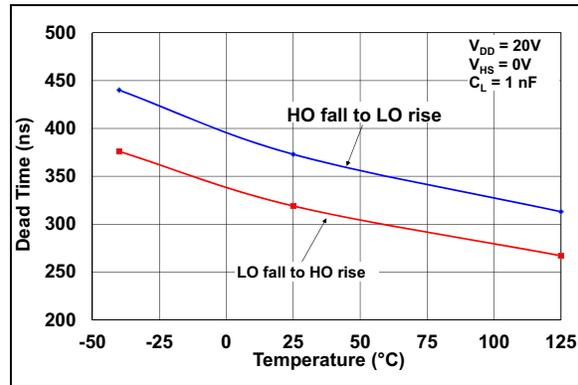
**FIGURE 2-30:** Dead Time vs. Temperature ( $V_{DD} = 20\text{V}$ ).
