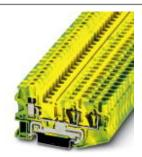
Feed-through terminal block, Connection type: Screw connection, Spring-cage connection, Cross section: 0.14 mm² - 6 mm², AWG :28- 12, Width: 6.2 mm, Color: green-yellow, Mounting: NS 35/7,5, NS 35/15
