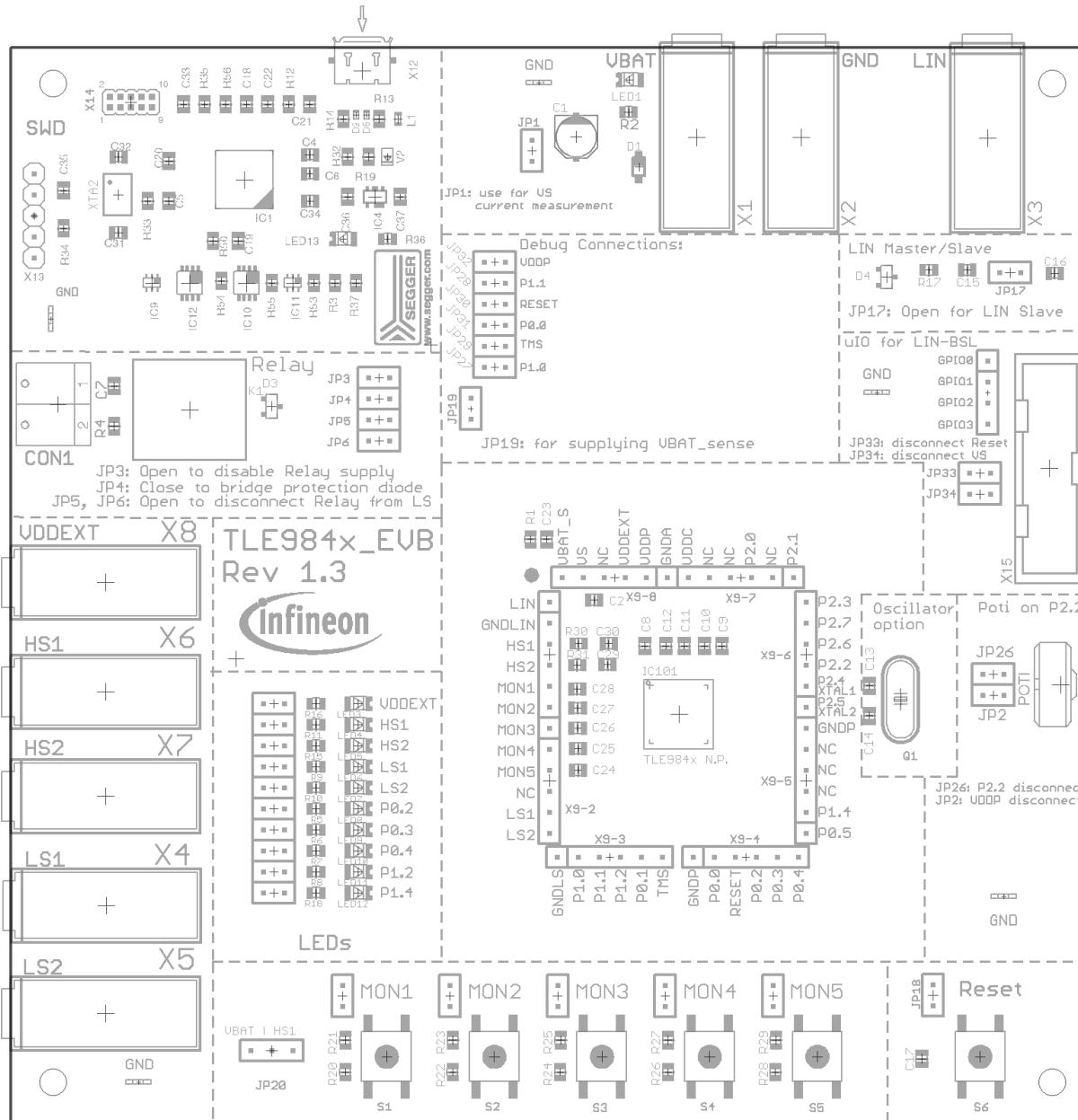
**Figure 8** Parts placement
