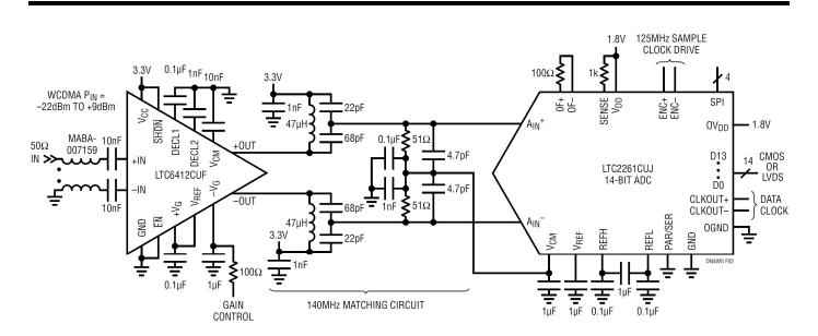
Figure 1. DC1600A Simplified Schematic
