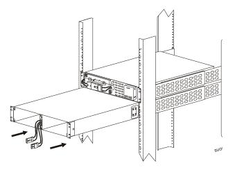
Secure the XLBP to the rack. Use two screws in each bracket.
