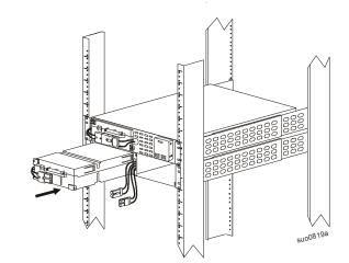
Secure the RBCs to the enclosure. Use three screws on each RBC.
