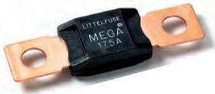
The MEGA® Fuse is designed for high current circuit protection up to 500A with "Diffusion Pill Technology." The MEGA® Fuse also provides time delay characteristics. Designed and patented by Littelfuse, the MEGA® Fuse is ideal for battery and alternator protection application and other heavy gauge cables requiring ultra-high current protection.
