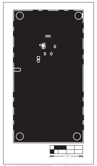
Figure 6. MAX4889A EV Kit PCB Layout—Solder Side
