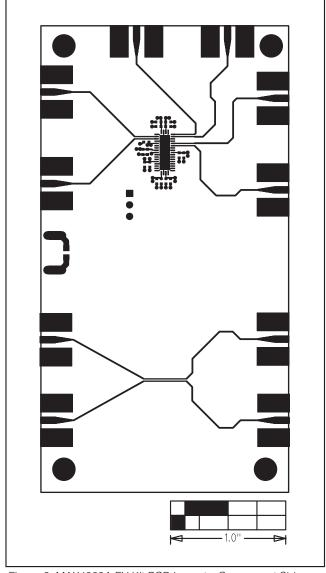
Figure 3. MAX4889A EV Kit PCB Layout—Component Side
