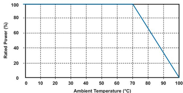
When the ambient temperature exceeds 70°C, reduce the rated power and current in accordance with the derating curve given
