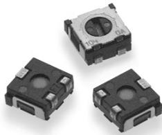
The 3204 miniature chip trimmer incorporates the latest technology developments and has been rigorously tested to the highest standards. Special attention during the design of the product, ensures that this component meets specific requirements of hybrids and modern surface mounting boards. It is fully sealed until you are ready to trim, so it is highly suitable for both dip and wave soldering. It can then be resealed by the use of rubber based lock paint.
