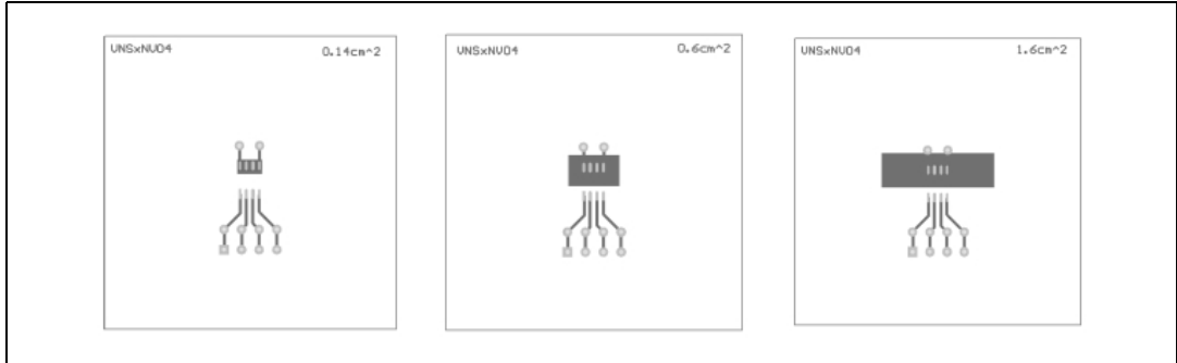
Figure 30. SO-8 PC board
