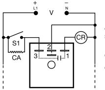
V = Voltage S1 = Initiate Switch, Contact, or Thermostat CR = Compressor Relay (Load) CA = Optional Cooling Anticipator
