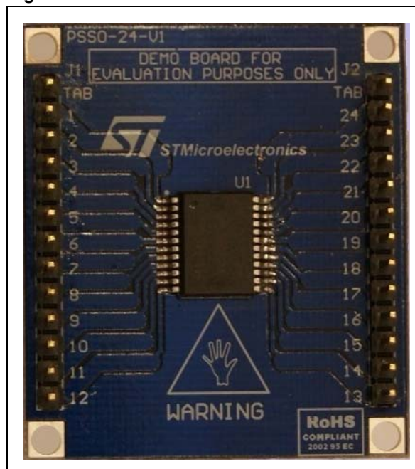
Figure 1. VND5E050K evaluation board
