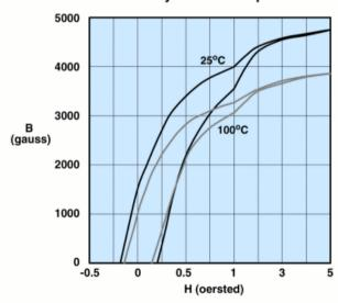
Measured on an 18/10/6mm toroid at 10kHz.
