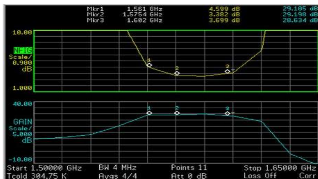
LNA Gain and Noise Figure @ 3.0V
