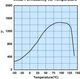
Measured on a 17/10/6mm toroid at 100kHz.
