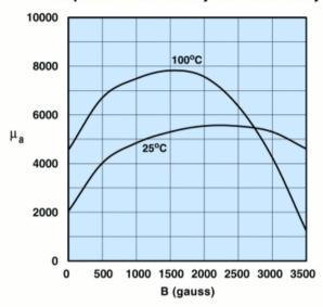
Measured on an 18/10/6mm toroid at 10kHz.
