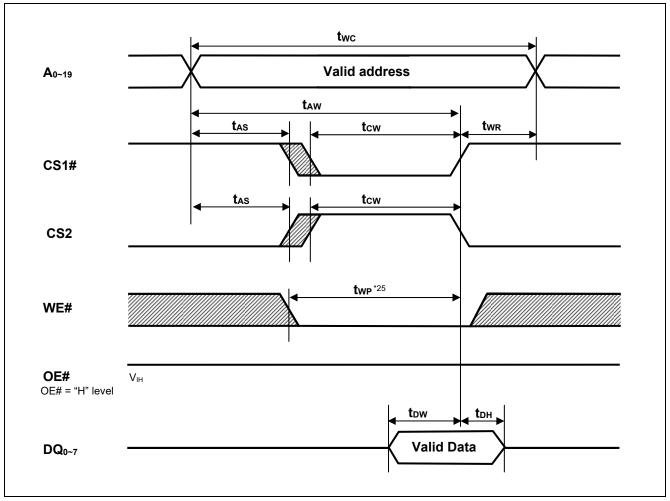
Note 25. twp is the interval between write start and write end.
