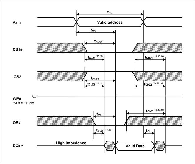
Note 14. t<sub>CHZ1</sub>, t<sub>CHZ2</sub> and t<sub>OHZ</sub> are defined as the time when the DQ pins enter a high-impedance state and are not referred to the DQ levels.
