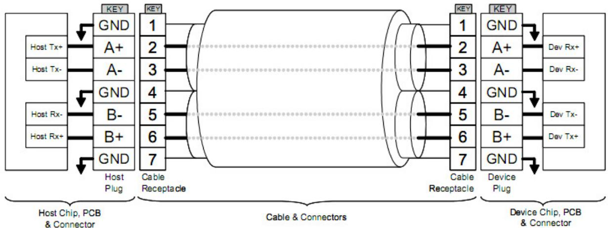
**Figure 3-2** SATA Cable / Connector Connection Diagram
