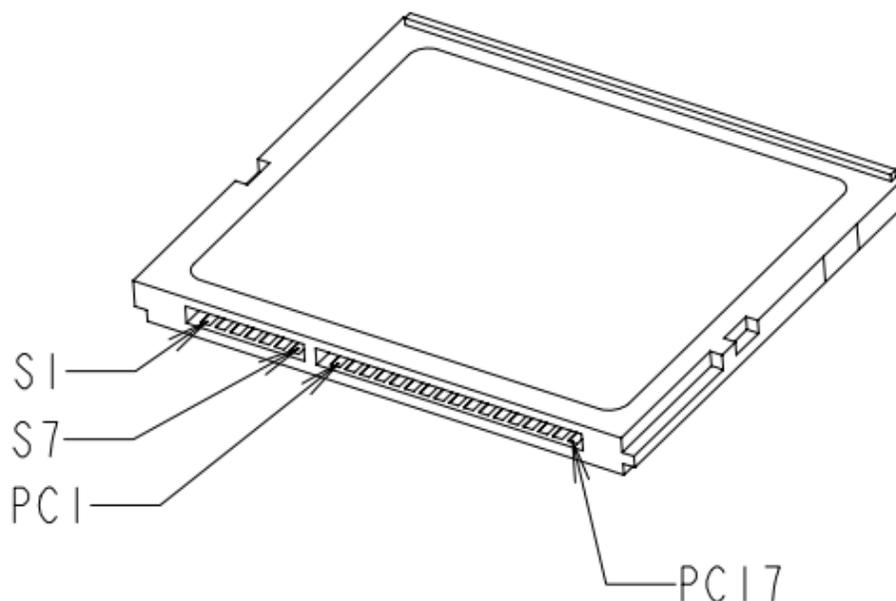
**Figure 3-1** Pin Assignment
