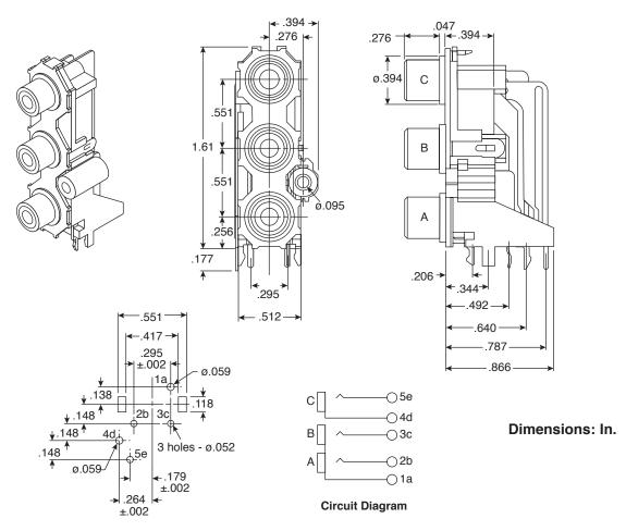
PCB Hole Layout (Bottom View)
