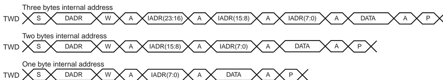
**Figure 30-12. Master Read with One, Two or Three Bytes Internal Address and One Data Byte**
