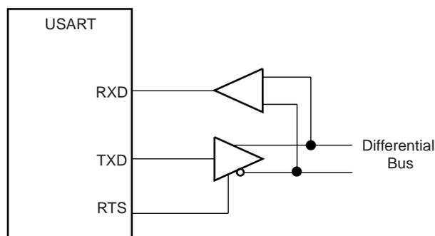
The USART is set in RS485 mode by programming the USART\_MODE field in the Mode Register (US\_MR) to the value 0x1.
