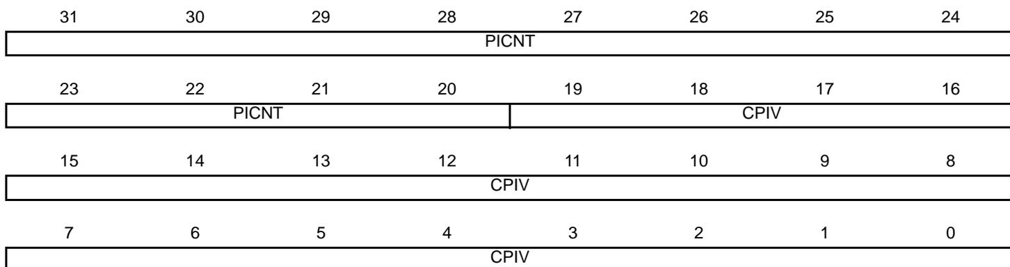
Reading this register clears PITS in PIT\_SR.
