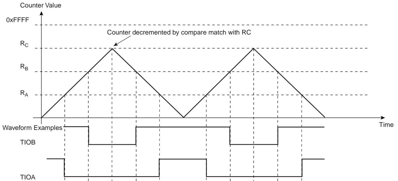
**Figure 33-14. WAVSEL = 11 With Trigger**
