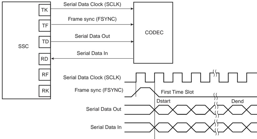
**Figure 32-19. Time Slot Application Block Diagram**
