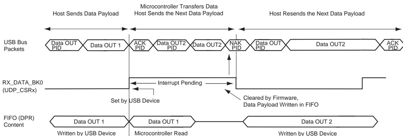
An interrupt is pending while the flag RX\_DATA\_BK0 is set. Memory transfer between the USB device, the FIFO and microcontroller memory can not be done after RX\_DATA\_BK0 has been cleared. Otherwise, the USB device would accept the next Data OUT transfer and overwrite the current Data OUT packet in the FIFO.
