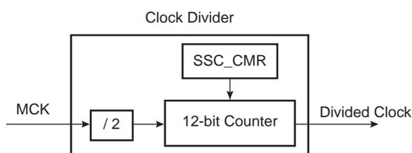
The Master Clock divider is determined by the 12-bit field DIV counter and comparator (so its maximal value is 4095) in the Clock Mode Register SSC\_CMCR, allowing a Master Clock division by up to 8190. The Divided Clock is provided to both the Receiver and Transmitter. When this field is programmed to 0, the Clock Divider is not used and remains inactive.
