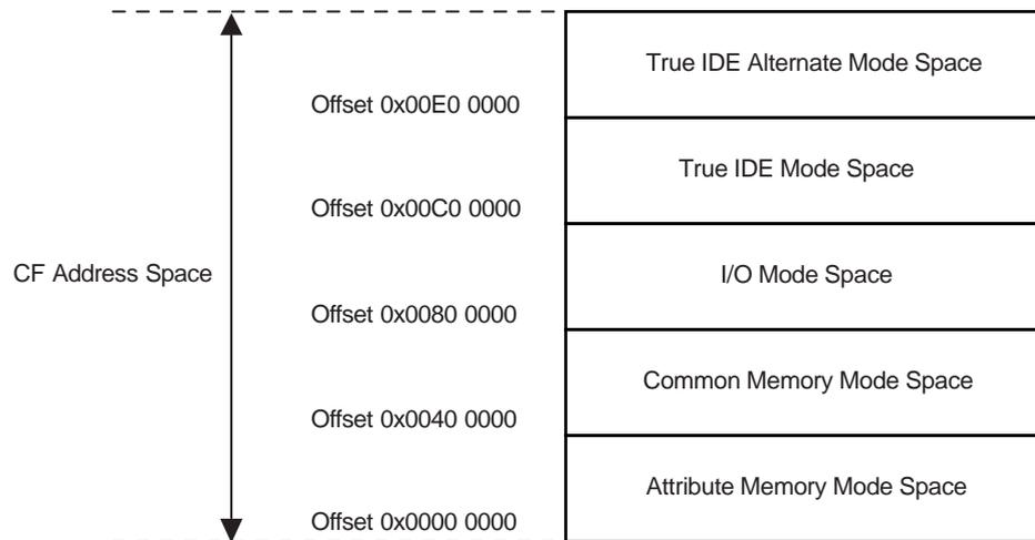
Note: The A22 pin of the EBI is used to drive the REG signal of the CompactFlash Device (except in True IDE mode).
