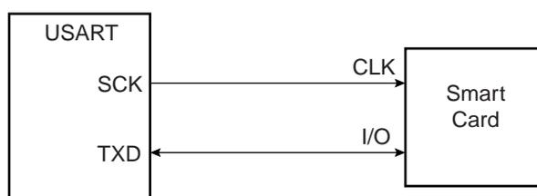
When operating in ISO7816, either in T = 0 or T = 1 modes, the character format is fixed. The configuration is 8 data bits, even parity and 1 or 2 stop bits, regardless of the values programmed in the CHRL, MODE9, PAR and CHMODE fields. MSBF can be used to transmit LSB or MSB first. Parity Bit (PAR) can be used to transmit in normal or inverse mode. Refer to [“USART Mode Register” on page 459](#) and [“PAR: Parity Type” on page 460](#).
