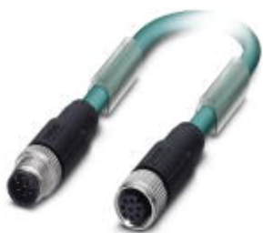
Assembled Ethernet cable, shielded, 4-pair, AWG 26 stranded (7-wire), RAL 5021 (sea blue), M12 plug to M12 socket, line, length 2.5 m
