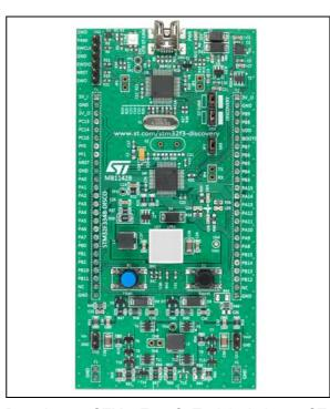
Based on an STM32F334C8T6, it includes an ST-LINK/V2-1 embedded debug tool interface, high brightness LED dimming with buck converter, buck/boost converter, LEDs and pushbuttons.
