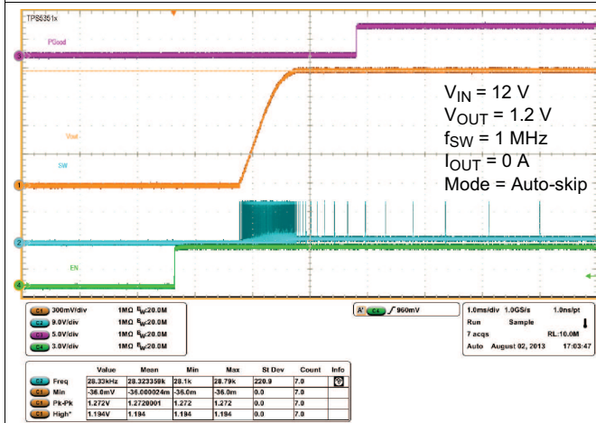
Figure 19. Auto-Skip Mode Load Transient
