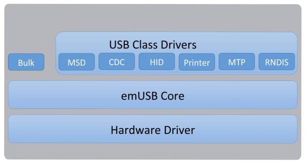
The different available hardware drivers, the USB class drivers, and the bulk communication component are additional packages, which can be combined and ordered as they fit to the requirements of your project. Normally, emUSB consists of a driver that fits to the used hardware, the emUSB core and at least one of the USB class drivers.
