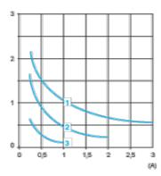
**DC-** Control of electromagnets (L/R  $\leq$  2 x (Ue x le) in ms, with Ue: rated operating voltage and le: rated operating current)
