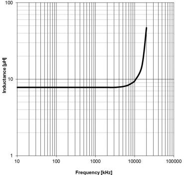
DESCRIPTION Projection **WE-WPCC Wireless Power Charging Receiver Coil** Würth Elektronik eiSos GmbH & Co. KG EMC & Inductive Solutions Max-Eyth-Str. 1 Order.- No. 74638 Waldenburg COMPLIANT SIZE Germany **RoHS&REACh** Tel. +49 (0) 79 42 945 - 0 WÜRTH ELEKTRONIK 760308102210 www.we-online.com A4 2014-03-24 SSt CSo 1.0 eiSos@we-online.com REV BY Size: 3737 DATE CHECKED
