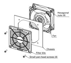
Replacement filters can be replaced by taking off the front part of the filter kit. There is no need to remove the screws.
