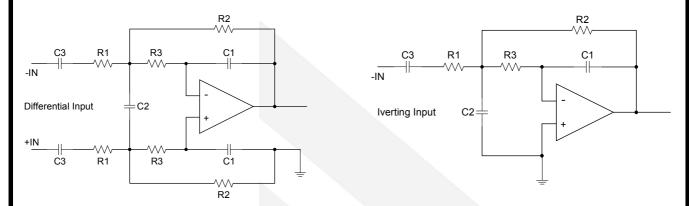
Figure 3 Second-Order Active Low-Pass Filter
