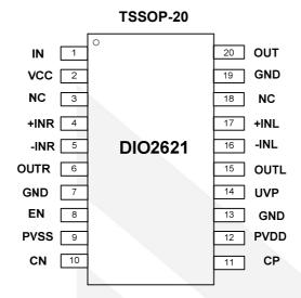
Figure 1 Pin Assignment
