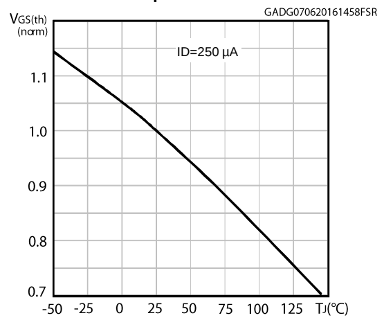
Figure 9: Normalized gate threshold voltage vs. temperature
