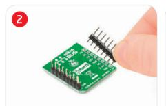
Turn the board upside down so that bottom side is facing you upwards. Place shorter pins of the header into the appropriate soldering pads.
