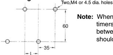
Note: When mounting two or more timers in line, dimension L between two adjacent timers should be 10 mm min.
