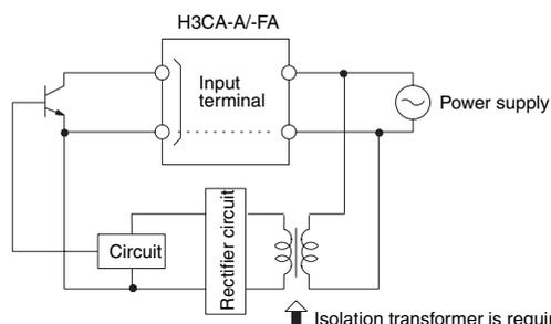
A transformer is not used in the power supplies for the H3CA-A and H3CA-FA. You can therefore receive an electrical shock by touching the input terminals when the power supply voltage is being applied. Take adequate precautions to protect against electrical shock.
