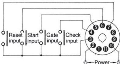
For each signal input contact, use a gold-plated contacts with high reliability. Be sure that these input signals satisfy the following requirements: a resistance of 1 kΩ (max.) and a residual voltage of 1 V (max.) when the contact is made.
