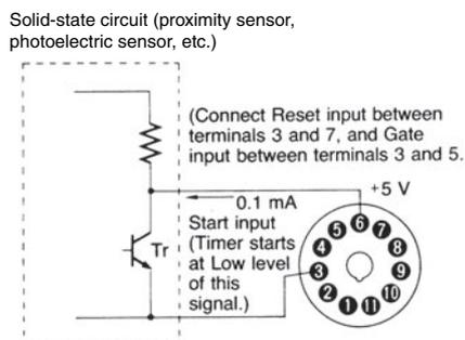
**Note:** Except for the power supply circuitry, avoid the laying of input signal wires in parallel or in the same conduit with high-tension or power lines. It is recommended to use shielded wires or wiring with independent metal conduits for the shortest possible distance.
