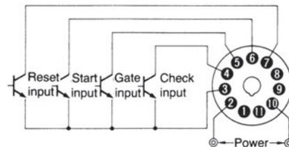
For signal input, use an open collector type transistor with characteristics:  $V_{CE0} = 20 \text{ V min.}$ ,  $V_{CE(S)} = 1 \text{ V max.}$ ,  $I_C = 50 \text{ mA min.}$  and  $I_{CBO} = 0.5 \mu\text{A max.}$  In addition, be sure that the input signals satisfy the following requirements: a resistance of 1 kΩ (max.) and a residual voltage of 1 V (max.) when the transistor is ON, and a resistance of 200 kΩ (min.) when the transistor is OFF.
