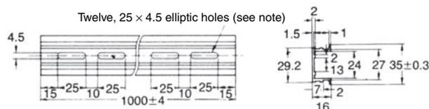
**Note:** A total of 12-25 × 4.5 elliptic holes are provided with 6 holes cut from each rail end at a pitch of 10 mm between holes.
