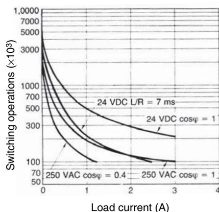
Reference: A maximum current of 0.15 A can be switched at 125 VDC (cosφ = 1).
