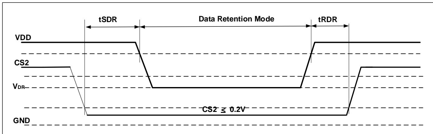
DATA RETENTION WAVEFORM (UB# AND LB# CONTROLLED)
