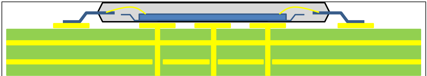
Figure 8-1: Example Thermal Via Holes on PCB.
