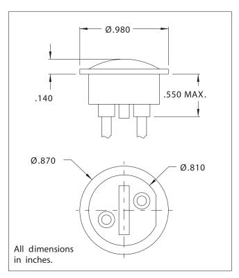
Mounting: Supplied with speednut SN2089. Mounting hole pattern on page SP2.
