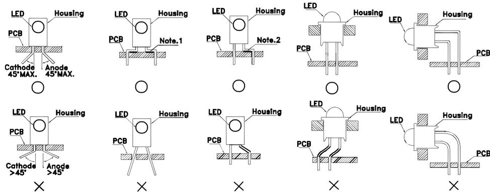
"○" Correct mounting method "×" Incorrect mounting method
