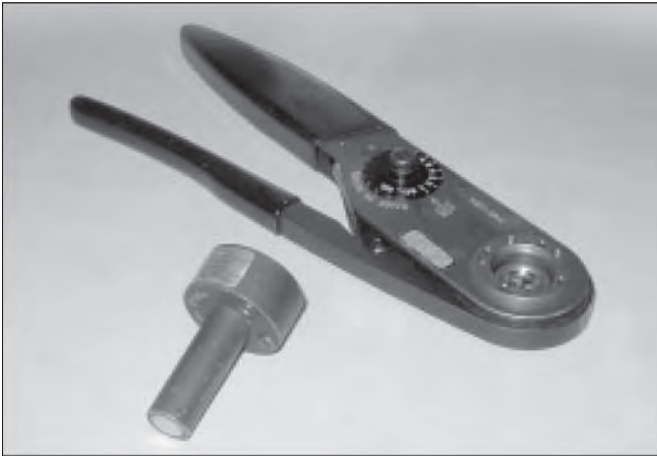
Crimp tooling M317 and locator VGE1 0077A
