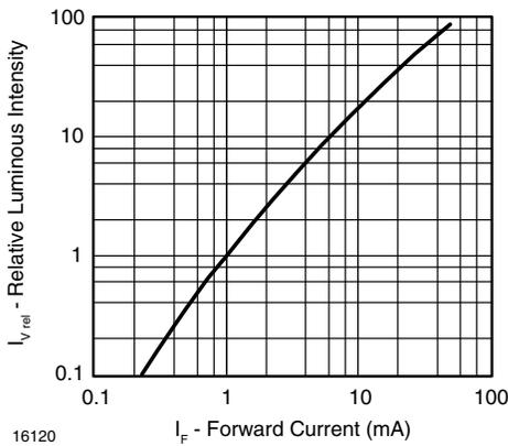
Fig. 4 - Relative Luminous Intensity vs. Forward Current
