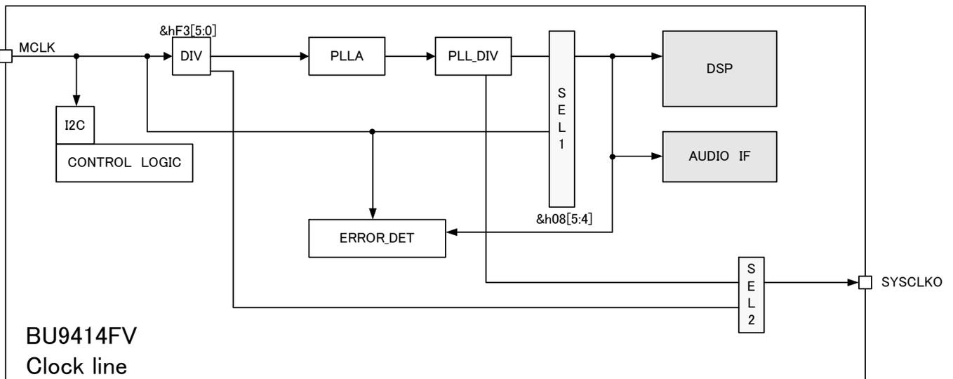
The clock system figure of BU9414FV is as mentioned above.
