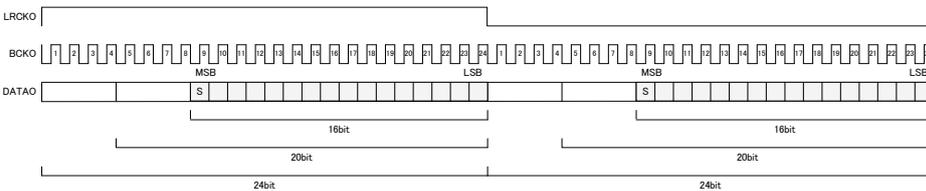
**3-1. Three-wire serial input's bit clock frequency setting**
