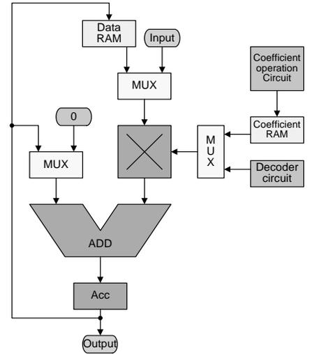
Digital signal from 16bit to 24bit is inputted to DSP, and it is extended by +8bit (+42dB) as overflow margin on the upper side. The clip process is performed in DSP when the process exceeding this range is performed.
