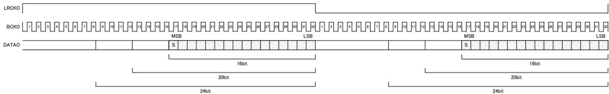
5-1. Format setting of three line serial output
