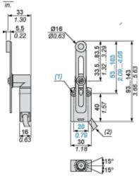
(1) 2 fixing holes  $\emptyset$  4.2 mm, counterbored  $\emptyset$  8 mm by 4 mm deep.
