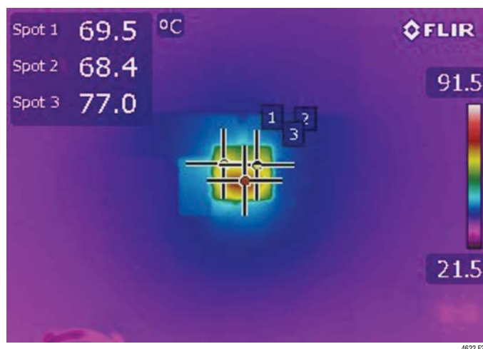
Figure 22. Thermal Picture, 12V Input, 3.3V and 5V Output, 2.5A DC Each Output with No Air Flow and No Heat Sink
