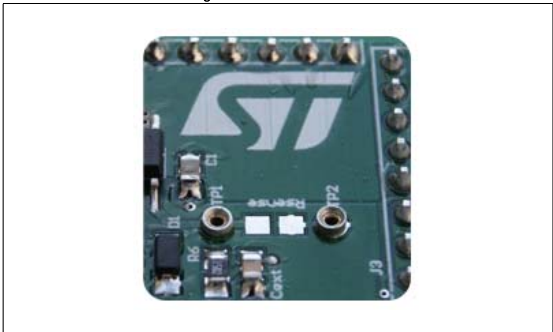
Figure 3. No sense resistor
