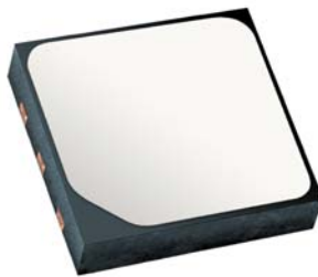
Figure 7. Si7021 with Factory-Installed Protective Cover
