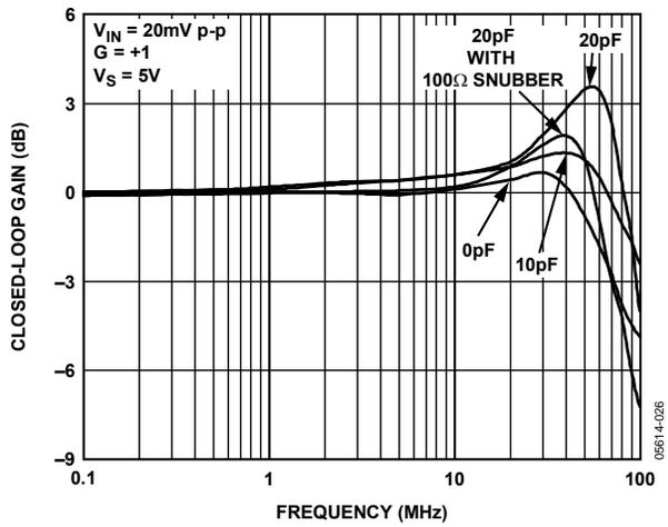
Figure 7. Small Signal Frequency Response vs. Capacitive Load
