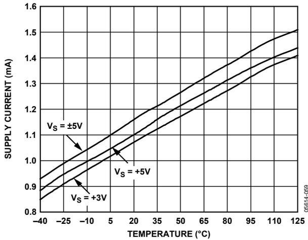
Figure 37. Supply Current vs. Temperature for Various Supplies
