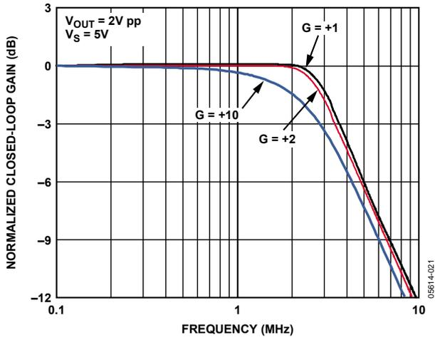
Figure 6. Large Signal Frequency Response vs. Gain
