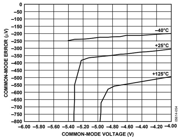
Figure 43. -CMV vs. Common-Mode Error vs.  $V_{OS}$
