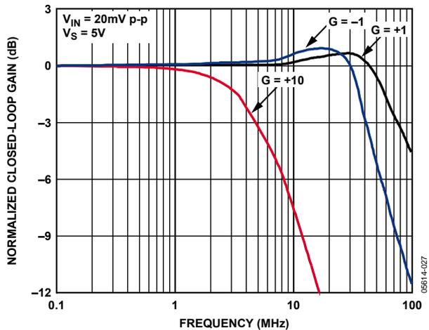
Figure 8. Small Signal Frequency Response vs. Gain
