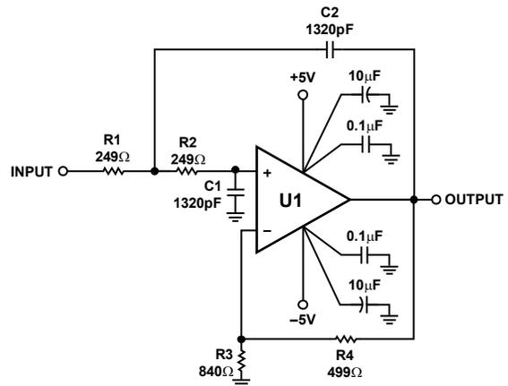
Figure 49. Two-Pole 500 kHz Reconstruction Filter Schematic
