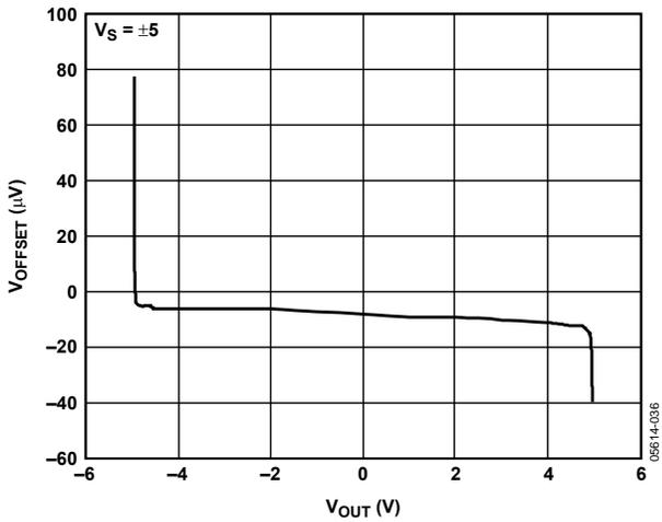
Figure 20. Input Error Voltage vs. Output Voltage
