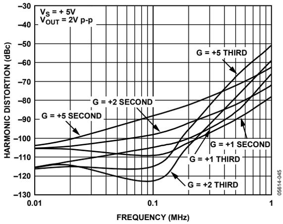
Figure 13. Harmonic Distortion vs. Frequency for Various Gains
