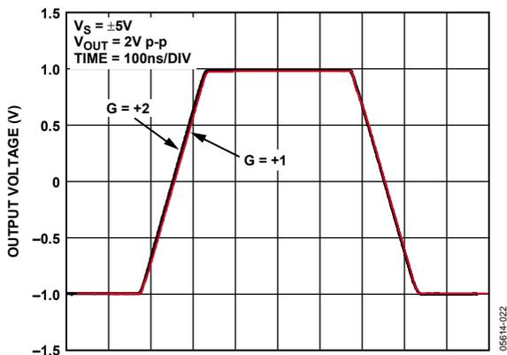
Figure 26. Large Signal Transient Response for Various Gains
