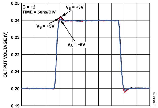
Figure 21. Small Signal Transient Response for Various Supplies
