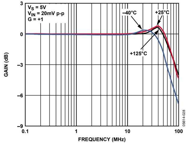
Figure 9. Small Signal Frequency Response vs. Temperature
