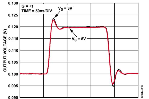
Figure 23. Small Signal Transient Response for Various Supplies
