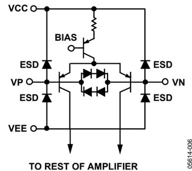
Figure 47. Input Stage and Protection Diodes
