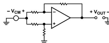
Figure 44. Common-Range Subtractor
