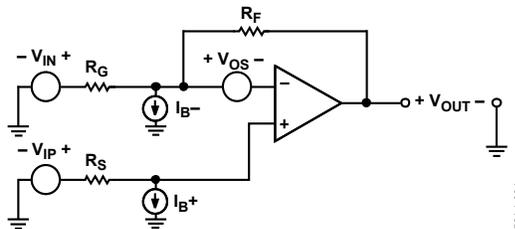
Figure 39. Typical Connection Diagram and DC Error Sources
