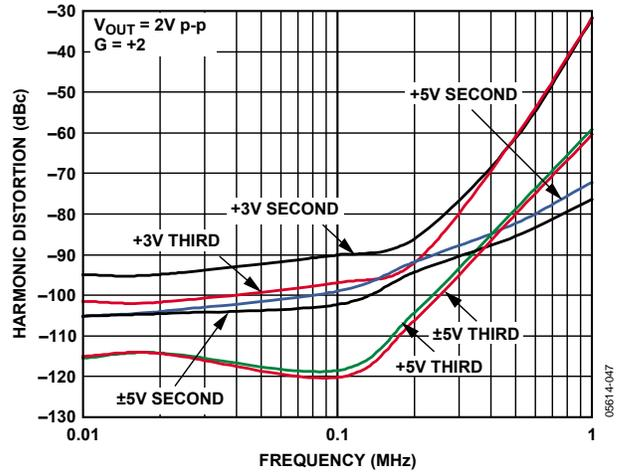
Figure 15. Harmonic Distortion vs. Frequency for Various Supplies
