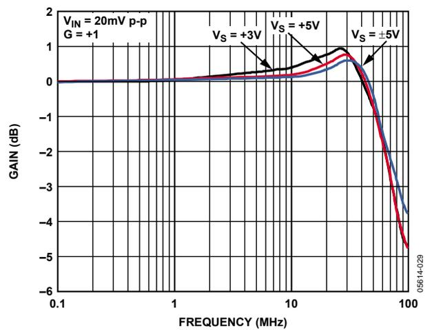
Figure 10. Small Signal Frequency Response vs. Supply Voltage
