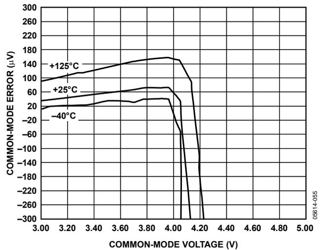
Figure 42. +CMV vs. Common-Mode Error vs.  $V_{OS}$
