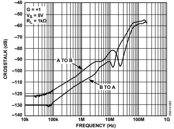
Figure 38. Crosstalk Output to Output
