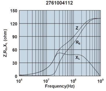
Impedance, reactance, and resistance vs. frequency.
