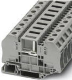
Test disconnect terminal block, With test socket screws for insertion of test plugs, Connection type: Bolt connection, Cross section: 0.1 mm<sup>2</sup> - 6 mm<sup>2</sup>, AWG: 26 - 10, Nominal current: 41 A, Nominal voltage: 500 V, Length: 82.4 mm, Width: 12.3 mm, Color: gray, Assembly: NS 35/7,5, NS 35/15
