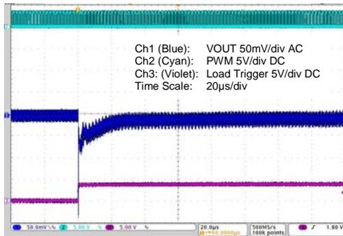
**Figure 4-34 20 to 5A Load Step – Min. Capacitance**
