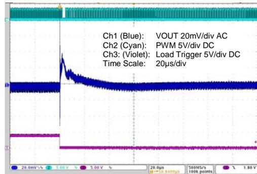
**Figure 4-20 5 to 15A Load Step – Max. Capacitance**
