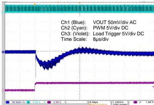
**Figure 4-31 20 to 5A Load Step – Max. Capacitance**
