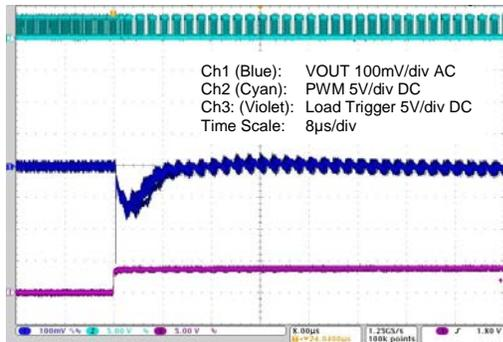
**Figure 4-24 20 to 5A Load Step – Min. Capacitance**
