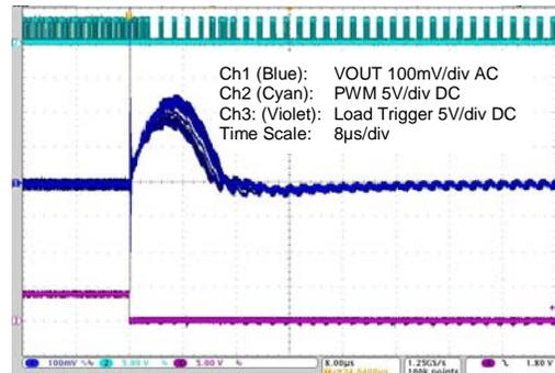
**Figure 4-5 5 to 15A Load Step – Max. Capacitance**
