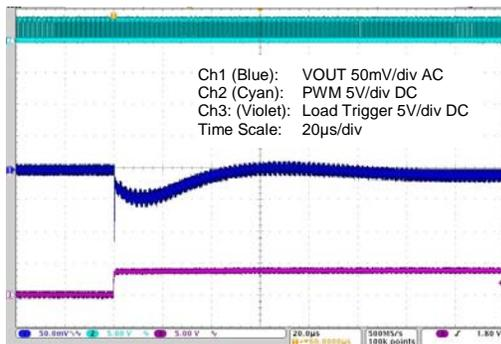
**Figure 4-36 20 to 5A Load Step – Max. Capacitance**
