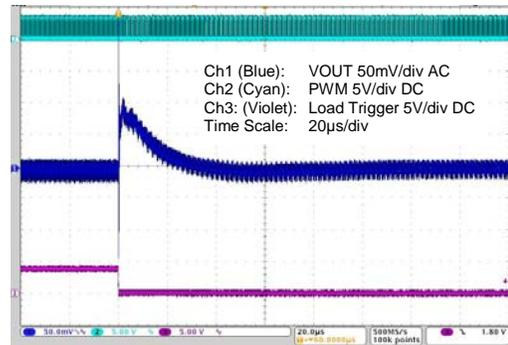
**Figure 4-35 5 to 20A Load Step – Max. Capacitance**
