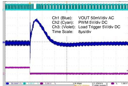
**Figure 4-30 5 to 20A Load Step – Max. Capacitance**
