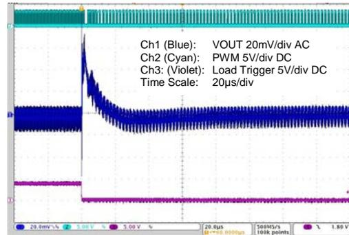
**Figure 4-15 5 to 15A Load Step – Max. Capacitance**
