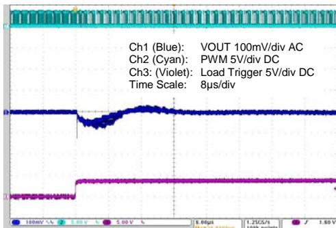
**Figure 4-6 15 to 5A Load Step – Max. Capacitance**
