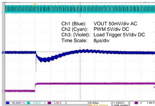
**Figure 4-11 15 to 5A Load Step – Max. Capacitance**
