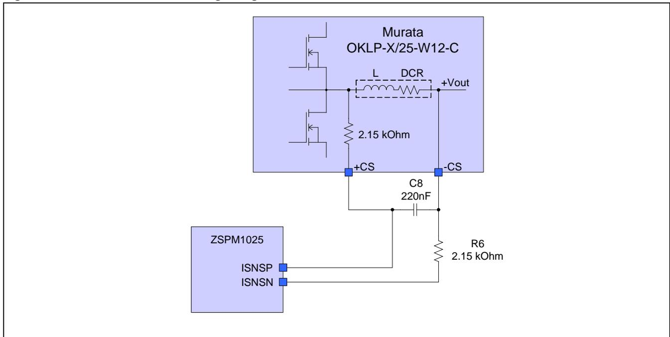
To improve the accuracy of the current measurement, which can be adversely affected by the temperature coefficient of the inductor's DCR, the ZSPM1025C/D features temperature compensation via the external temperature sensing. The temperature of the inductor can be measured with an external temperature sense element placed close to the inductor. This information is used to adapt the gain of the current sense path to compensate for the increase in actual DCR.
