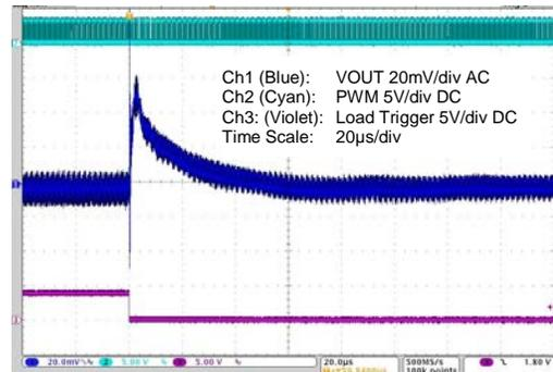
**Figure 4-40 5 to 20A Load Step – Max. Capacitance**
