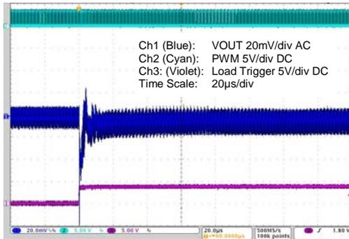
**Figure 4-14 15 to 5A Load Step – Min. Capacitance**
