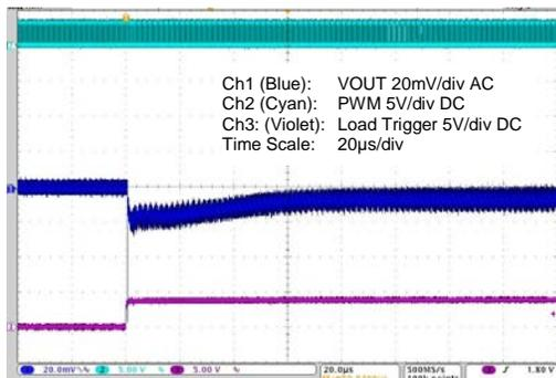
**Figure 4-41 20 to 5A Load Step – Max. Capacitance**
