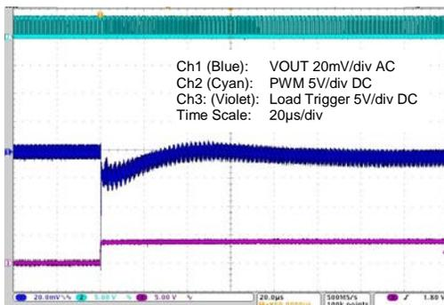
**Figure 4-16 15 to 5A Load Step – Max. Capacitance**
