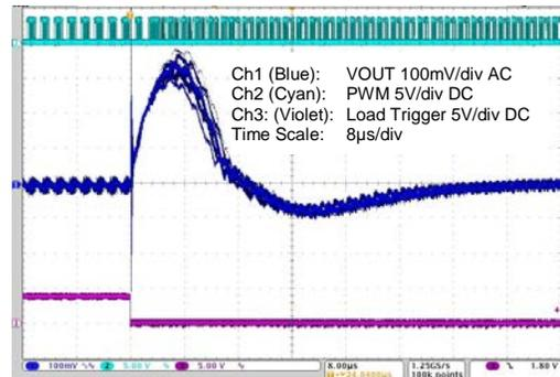
**Figure 4-25 5 to 20A Load Step – Max. Capacitance**
