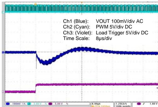
**Figure 4-26 20 to 5A Load Step – Max. Capacitance**
