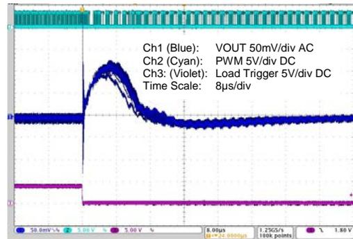
**Figure 4-10 5 to 15A Load Step – Max. Capacitance**
