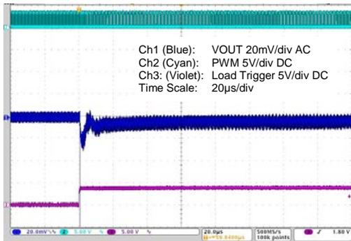
**Figure 4-19 15 to 5A Load Step – Min. Capacitance**
