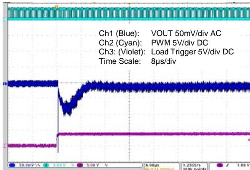
**Figure 4-29 20 to 5A Load Step – Min. Capacitance**
