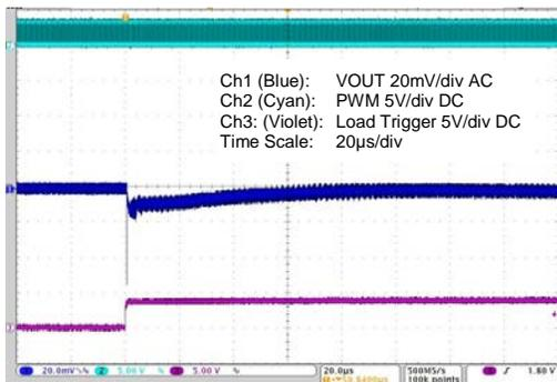
**Figure 4-21 15 to 5A Load Step – Max. Capacitance**
