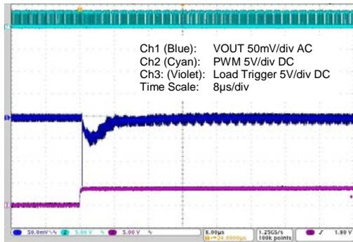
**Figure 4-9 15 to 5A Load Step – Min. Capacitance**
