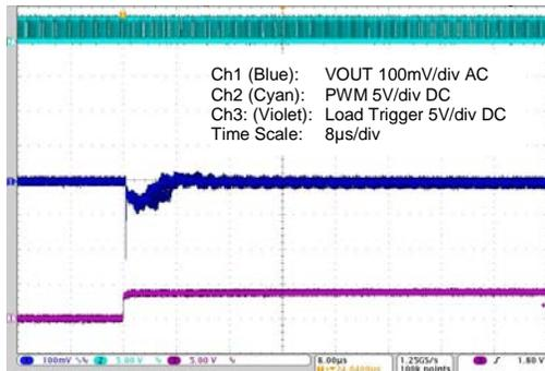
**Figure 4-4 15 to 5A Load Step – Min. Capacitance**
