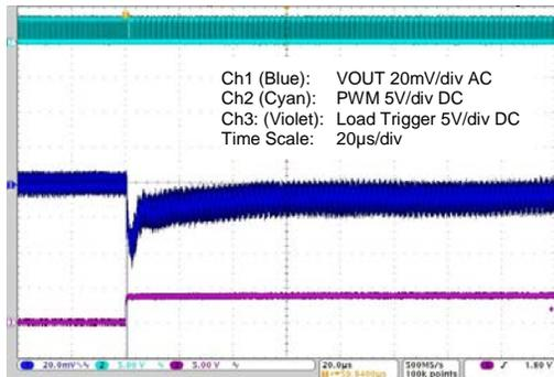
**Figure 4-39 20 to 5A Load Step – Min. Capacitance**
