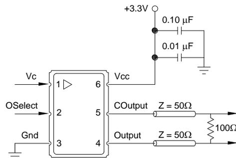
**LVDS to LVDS:** The 100 Ω resistor should be removed if this load is provided internally within the LVDS receiver.
