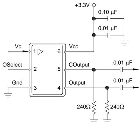
**Functional Test:** Allows use of standard power supply biasing configuration. Pull down resistors are used for LV-PECL outputs and are removed for LVDS outputs. Since the LVDS outputs are AC coupled, the output DC levels cannot be measured.
