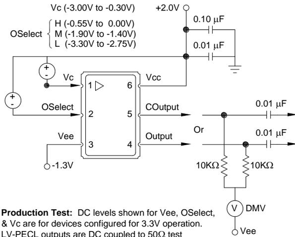
**Production Test:** DC levels shown for Vee, OSelect, &  $V_C$  are for devices configured for 3.3V operation. LV-PECL outputs are DC coupled to 50 Ω test equipment. LVDS outputs are connected to a digital volt meter, then AC coupled to the test equipment. The digital volt meter allows for Mid Level & Swing measurements.
