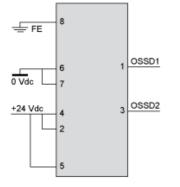
With External Device Monitoring (EDM) feedback loop
