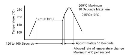
The part may be reflowed 2 times without degradation (typical for lead free processing).
