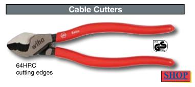
Cable Cutters Light, energy-saving & clean cutting with specially ground precision cutting edges. Long life is achieved through additional induction hardening of cutting edge to 64HRC. C70 special tool steel hardened and tempered. Soft vinyl grips. For cutting of copper & aluminum cables without crushing, also suitable for stripping. Not for steel cable, wires and copper conductors with hard coatings.
